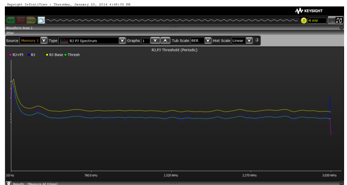
The RJ/PJ threshold tools, provides more jitter analysis
