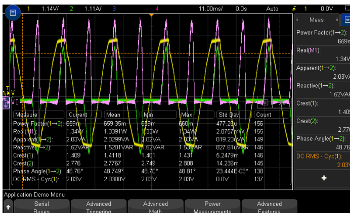
Figure 29a: Integrated power measurements make quick work of analyzing power producing and power consuming devices
