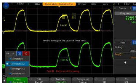
Figure 5: See up to four annotations on screen at once for documentation. The standard touch screen makes inputting notes simple.
