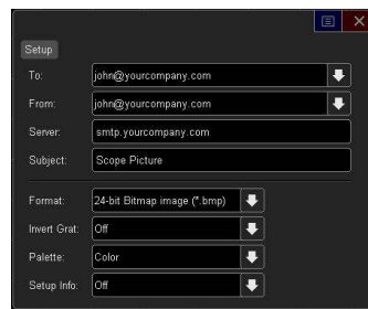
Figure 6: With the optional LAN/VGA module you can email yourself setups, data and screenshots.
