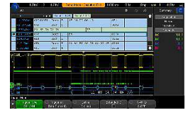
Figure 19: Multi-bus time aligned decode
