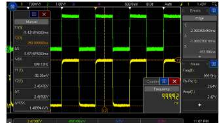
Figure 3: Side bar with movable docks allows information to be placed on the screen precisely where you want it for documentation.
