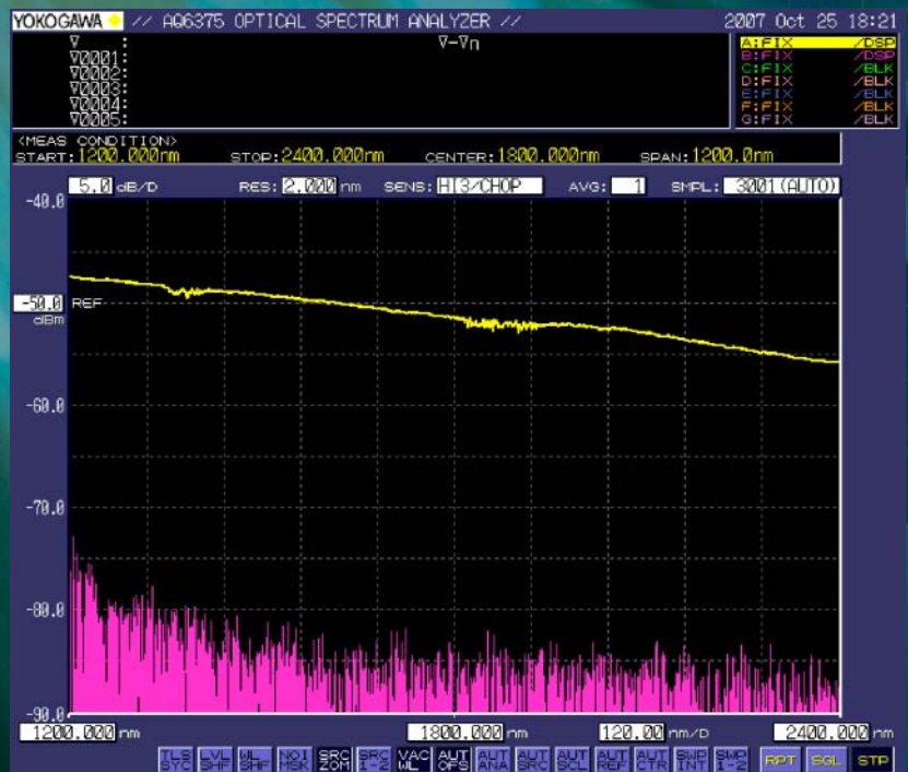
The spectrum of a white light source (yellow) and the background noise of AQ6375 (red)
