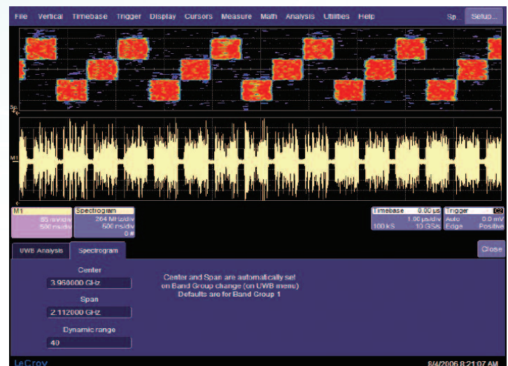
Spectrogram of a UWB signal hopping over three frequency bands of a band group.
