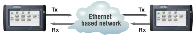
Running Service Activation Test in local - remote configuration using two MT1000A testers
