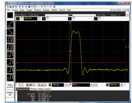
Figure 5. 100 ps pulse with 17 ps risetime.
