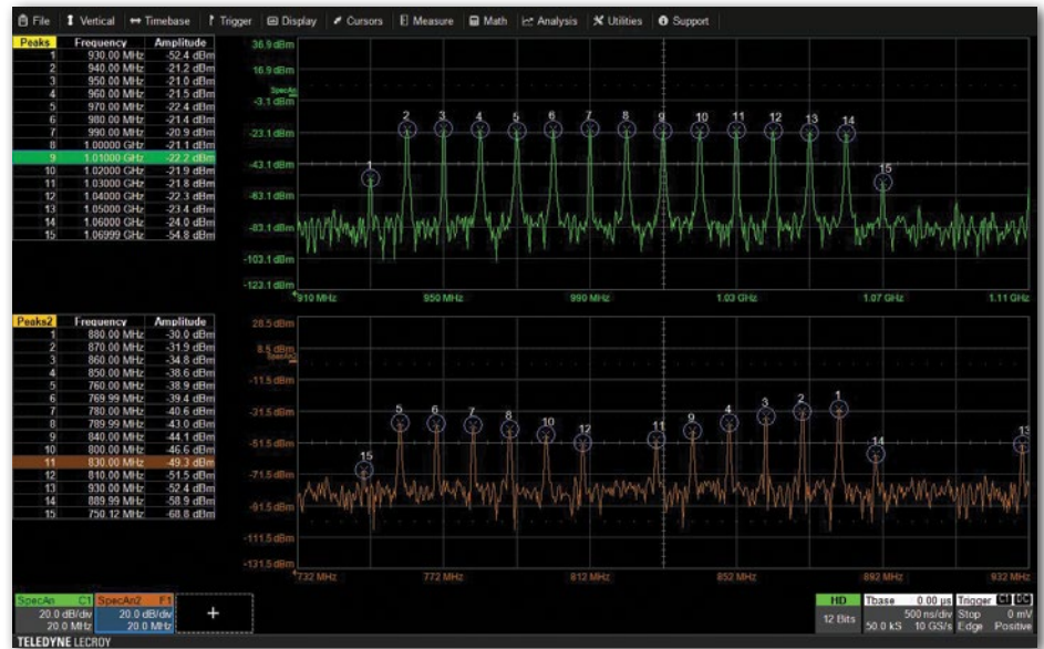
Use two independent input settings and frequency ranges for advanced spectrum analysis.
