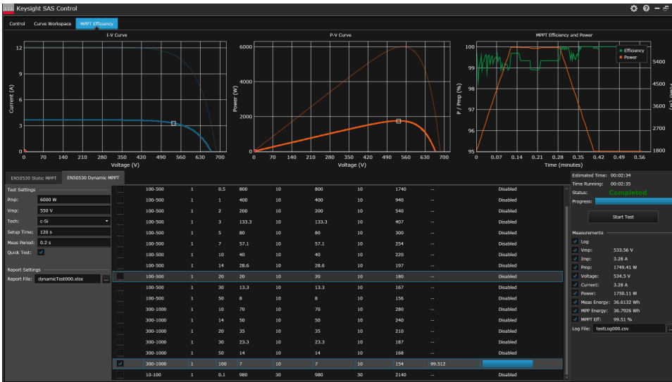
Figure 9. SAS Control Software performing dynamic EN50530 MPPT test
