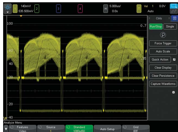
Figure 26: Triggering on 1080p HDTV signal analysis.
