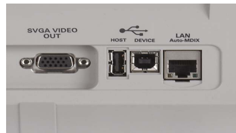
Figure 35: Standard VGA output, USB host and device and LAN.
