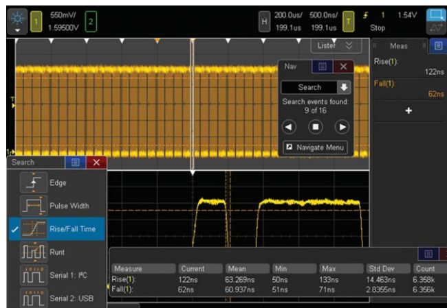
Figure 10: The 4000 X-Series was set up to capture data signals with various rise time edges. Using the search and navigation capability, the oscilloscope was able to find, mark (white triangles), and quickly navigate to 16 occurrences of “out of compliance” rise-time edges.
