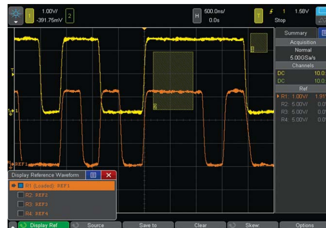
Figure 32: Store and recall up to four reference waveforms.
