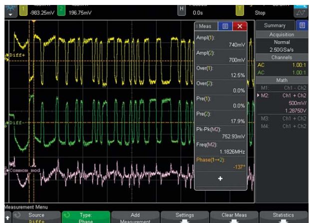
Figure 23: Dual channel WaveGen output of differential arbitrary signals. Common mode is shown as a math function.
