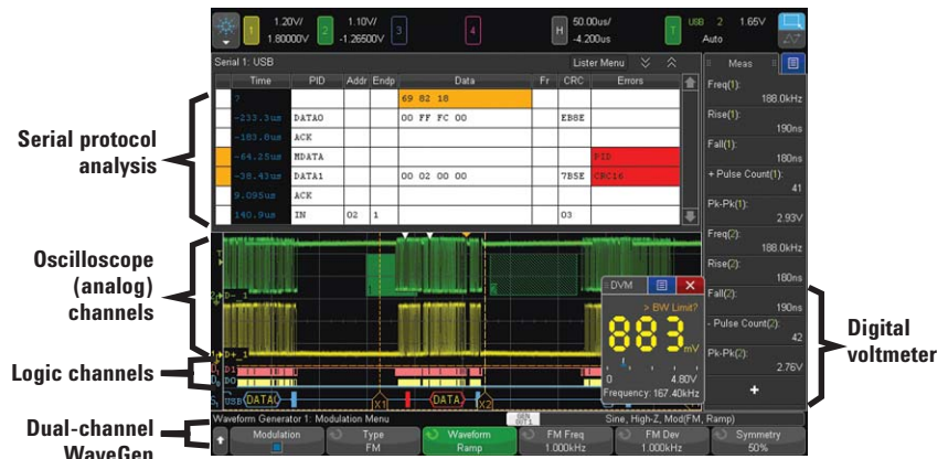
Figure 17: The 4000 X-Series provides the capabilities of five instruments seamlessly integrated into one.
