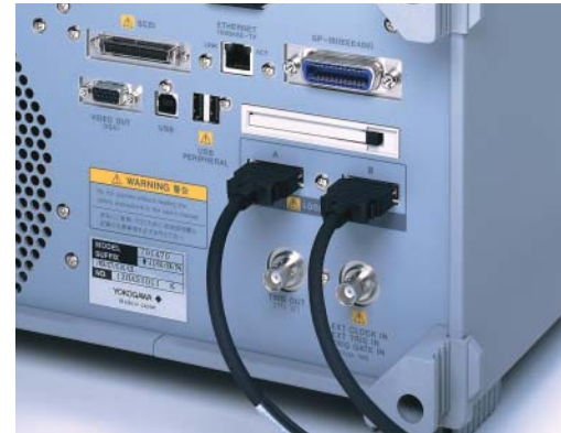
Example of Logic Probe Connection
