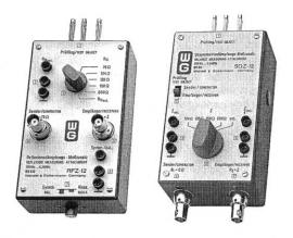
Both the SDZ-12 and the RFZ-12 have a connector for external standard impedances which can differ from the characteristic impedances normally used. The RN-120 standard impedance can be used to allow return loss measurements on the balanced 120  $\Omega$  connections to digital multiplexers.
