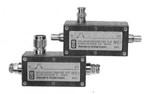
The RFZ-1 Bridge allows return loss measurements in the frequency range from approximately 50 kHz up to 180 MHz. It is available with 75  $\Omega$  or 50  $\Omega$  characteristic impedance.
