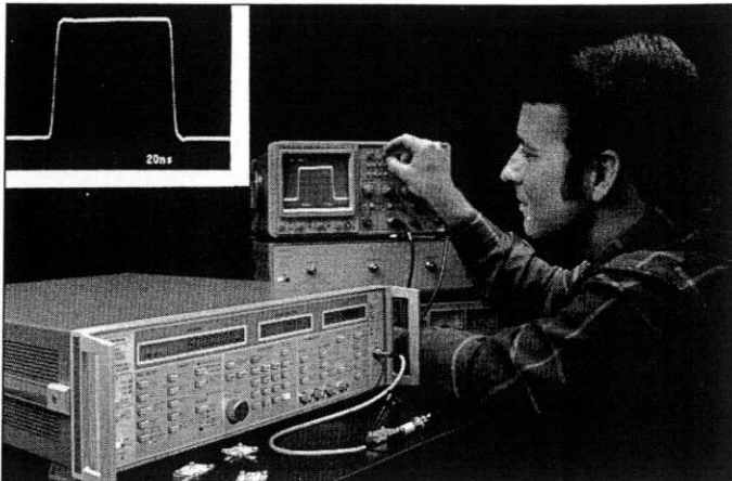
Built-in pulse generator typically has less than 5 ns rise time over a 25 ns to 99 ns pulse width range.
