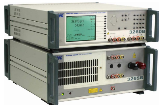
3265B DC Bias Unit can deliver up to 25 A of DC bias current in steps of 25 mA
