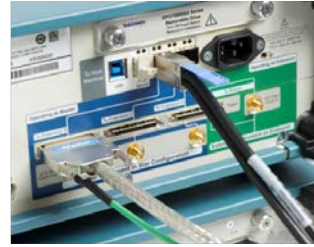
UltraSync connection on instrument with Master role
