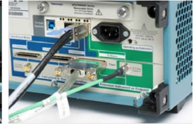
UltraSync connection on instrument with Extension role
