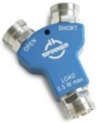
Calibration Kits for one-port measurements
