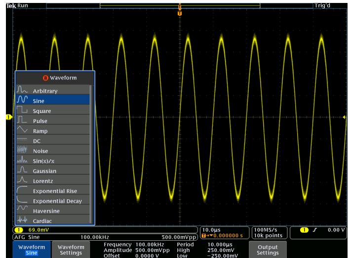
Waveform type selection in the integrated AFG.
