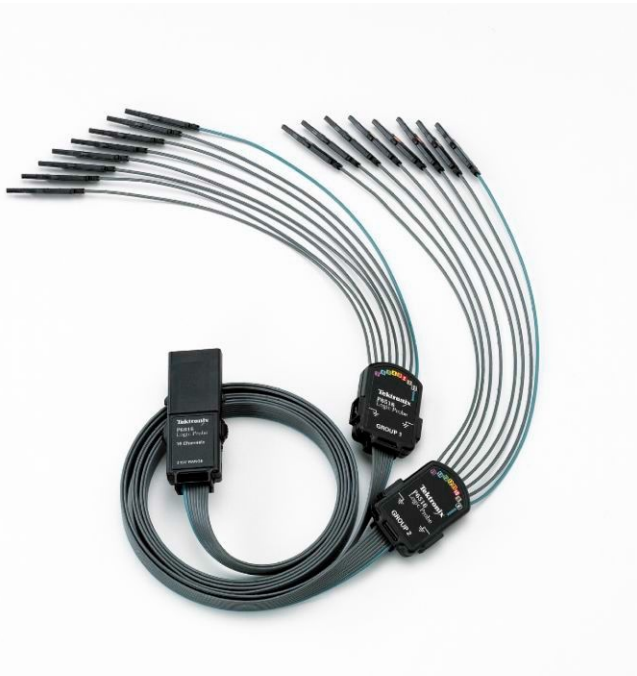
The P6616 MSO probe offers two eight-channel pods to simplify connecting to your device.
