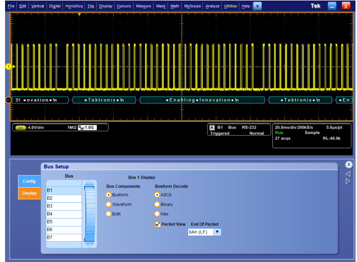
Packet View display of decoded RS-232 messages.
