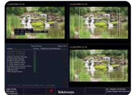
► Safe Action, Safe Title Graticules and Closed Caption and V-Chip Information shown in the picture display.
