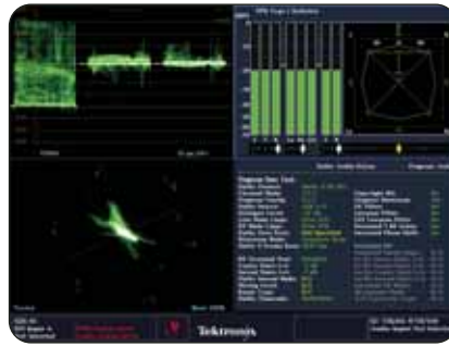
► Dolby E signal monitoring with multi-channel Surround Sound display and metadata analysis display.
