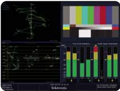
► Lightning display showing correctly aligned signal.
