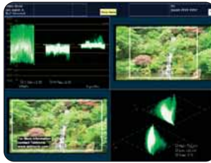
► Figure 8. Picture display with Closed Caption, Safe area graticules and gamut brightups.
