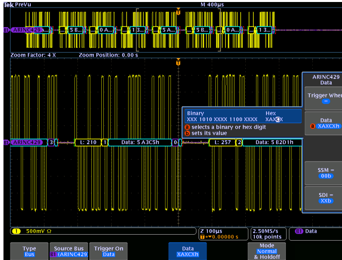
Triggering on a specific data value on the ARINC 429 bus.
