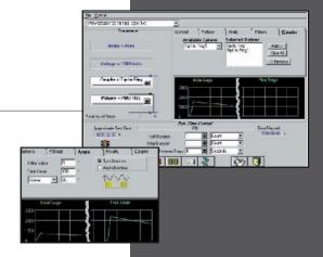
Optional WIN 2050 test management software offers Windows-based control of the pulse generator and access to a range of parameter selection, test sequencing, editing and reporting tools. The equipment-under-test is monitored electronically and repeated tests can be performed automatically. The built-in report generator automatically creates comprehensive files of test parameters and results, including manually selected coupling modes, ready for inclusion in a compliance report.
