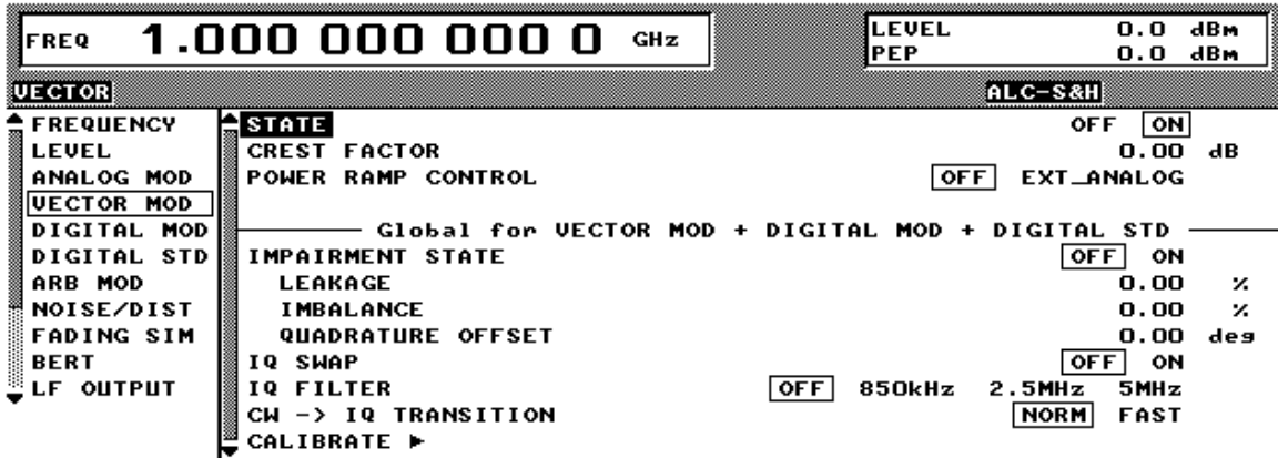
Fig. 2-34 VECTOR MOD menu (preset settings), equipped with option SMIQB47 and IQMOD var. 8 or higher
