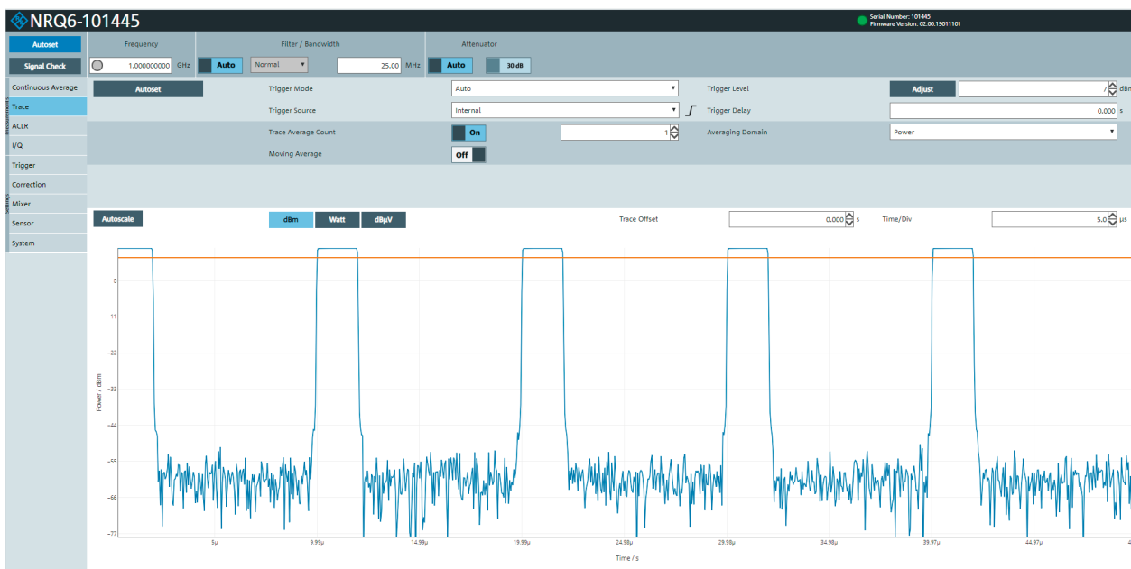
Trace measurement on a pulsed signal
