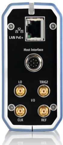
Rear view of the R&S®NRQ6 with hardware interfaces
