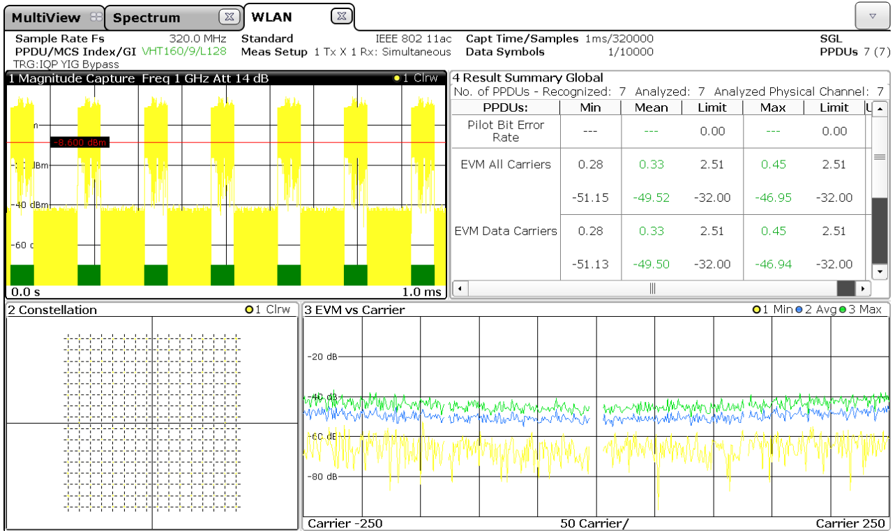
Measured EVM for an IEEE 802.11ac signal with 160 MHz bandwidth.
