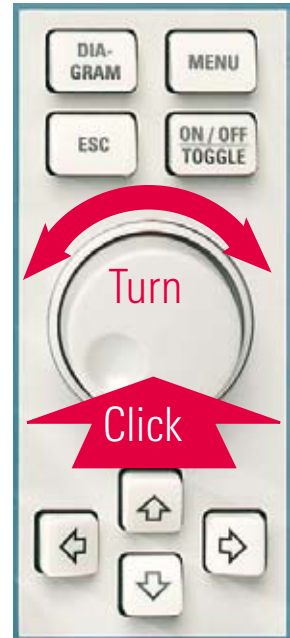
Rotary knob for navigation in the menus
