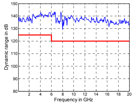
Dynamic range in dB versus frequency for the R&S®ZNB20.
