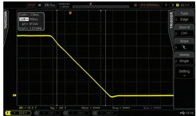
DC Voltage Ramp Down @ 100Vdc/ms programmed slew rate Captured
