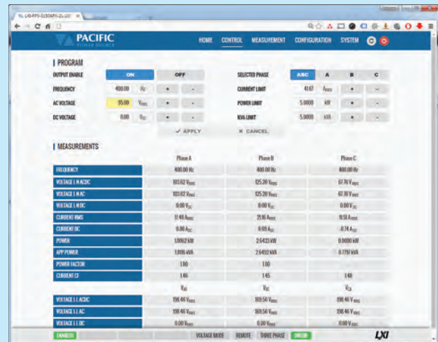
Control and Measurements Page shows settings and read backs
