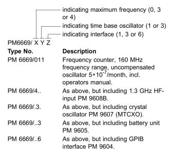
Example: PM 6669/416 means a PM 6669 frequency counter, including both an 160 MHz and an 1.3 GHz input channel, an uncompensated oscillator and a GPIB interface.
