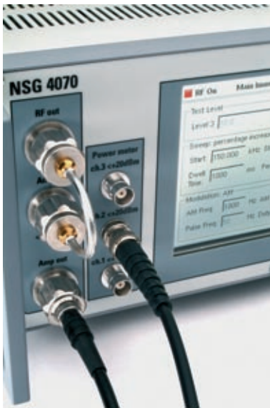
NSG 4070 front panel with RF ports
