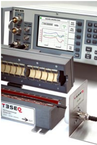
Application for IEC/EN 61000-4-6, calibration set-up with CDN
