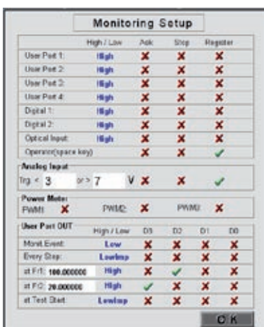
Software: EUT monitoring setup
