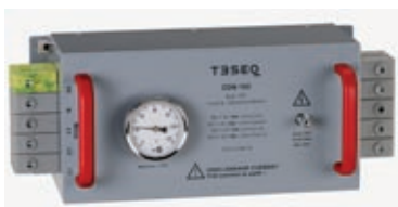
CDN 163, Burst Coupling Network 100A per channel
