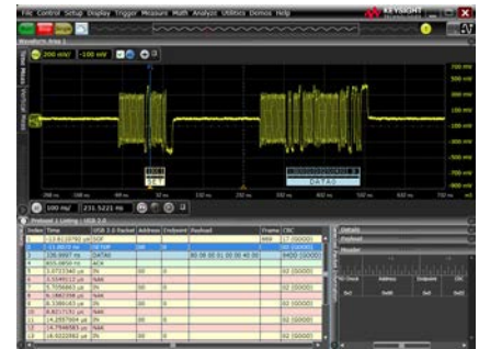
Trigger on and decode USB packets.
