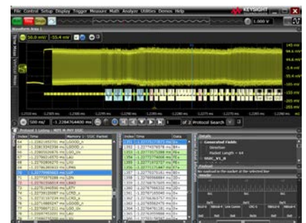
Trigger on and decode MIPI packets.
