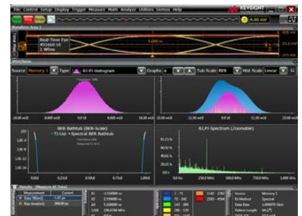
Analyze jitter plus RJ/DJ separation.
