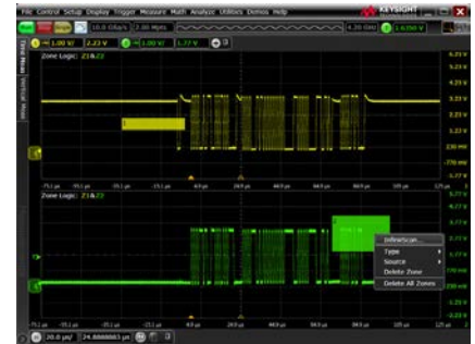
Identify signal integrity issues with InfiniiScan Zone – Qualify triggering.
