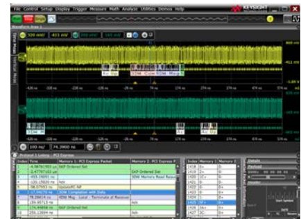
Trigger on and decode PCIe serial packets.
