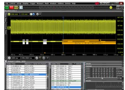
Trigger on and decode SATA serial packets.
