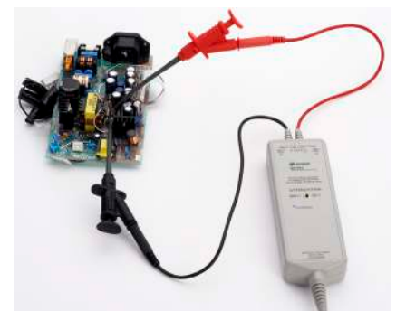
N2790A measuring a power supply signal
