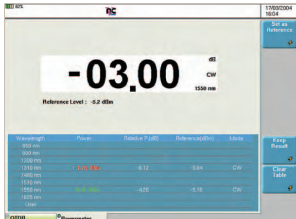
Jumper loss measurement
