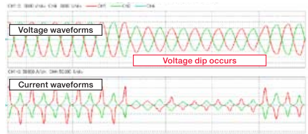
Voltage and Current Waveforms at the Time Voltage Dip Occurs
