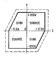
Sink current is limited to a value ranging linearly from .5A @ 0V to .25A @ 100V.
