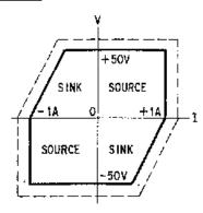
Sink current is limited to a value ranging linearly from 1A @ 0V to .5A @ 50V.
