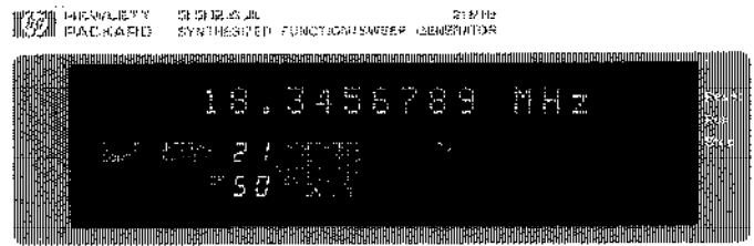
The sweep menu allows you to set up sweep parameters for each individual interval.
