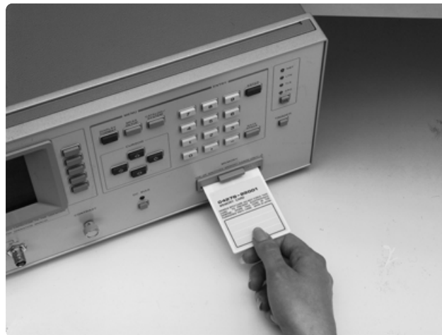
Inserting the memory card 1
