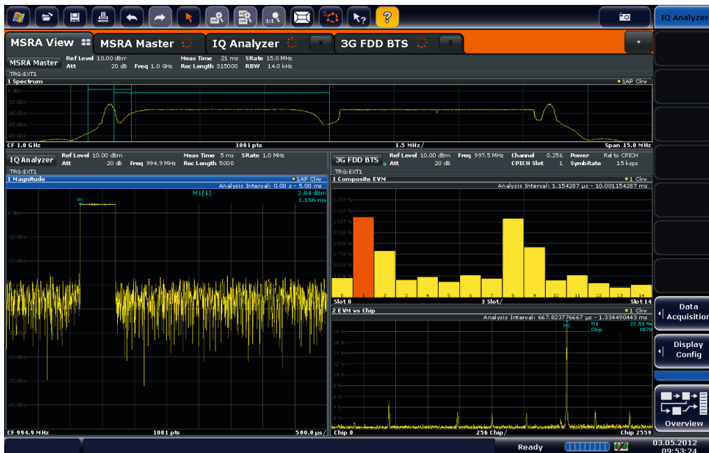
Multistandard radio analyzer (MSRA): Signals are captured once, then analyzed according to different standards and at different frequencies in parallel.
