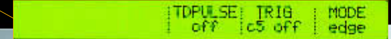
Fast edge rise time to 150 ps makes the 5820A well suited for oscilloscopes up to 2 GHz. A tunnel diode pulser drive mode makes it easy to work with even faster edges.
