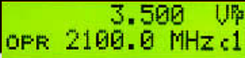
Leveled sine wave source to 600 MHz, extendible to 2.1 GHz, for calibrating bandwidth.
