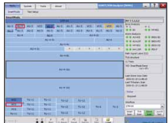
■ FTB-8120NGE/8130NGE SmartMode: multichannel signal discovery with real-time alarm scan (shown in the FTB-400 user interface).
