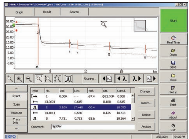
EXFO's FTB-7000D OTDR easily tests through high-port-count splitters with high loss levels.
