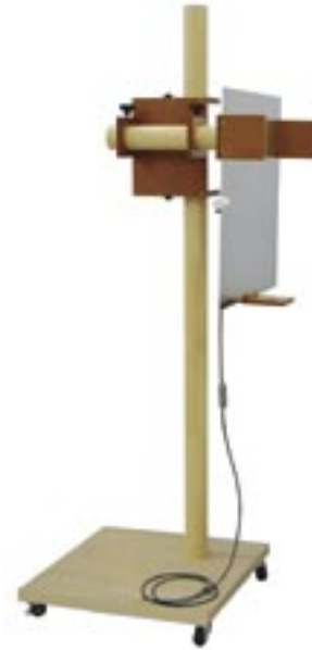
ESS-801GL (Vertical coupling plane & Cable with resistors)
