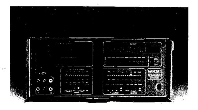
General View of Datron 4708 Autocal Multitunction Standard
