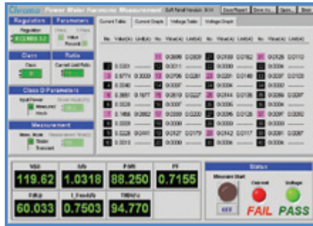
IEC 61000-3-2 Current Harmonic Test
