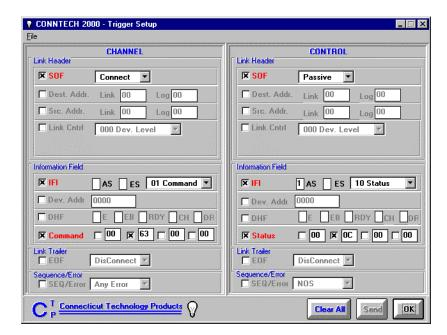
The **Analyzer** features a high level interface for defining the Trigger pattern for each trigger machine. Triggers are specified in terms of the logic of the protocol. A bit-level understanding of the protocol is not required to use the ConnTech 2000–ESC.
