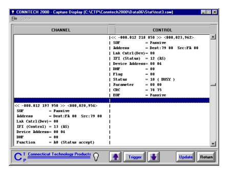
The **Analyzer** displays the Captured data in a format that is both easy to read and understand. Each frame is time stamped relative to the Trigger Point. The number of idles between frames is also displayed. The example above shows Control Unit Status being reported to the Channel.
