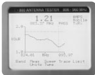
Swept frequency mode reveals a comprehensive picture of antenna matching.
