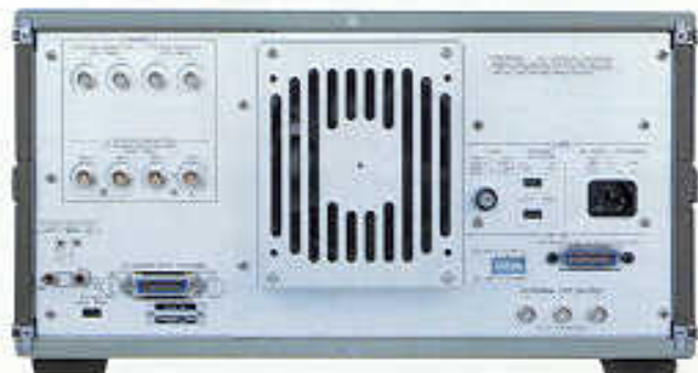
4145A Rear Panel includes 4 triax connectors for SMUs, 2 each BNCs for V_s and V_m , 16058A test fixture connector, and HP-IB connector.
