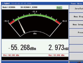
N9340B supports Meter and Chart mode to display the results of power measurements.
