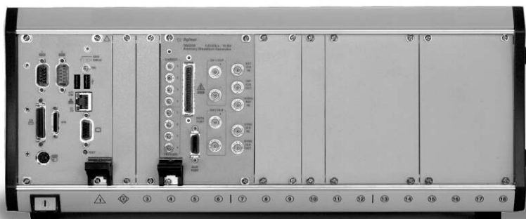
Figure 11. Agilent N6030A AWG with controller in CompactPCI chassis
