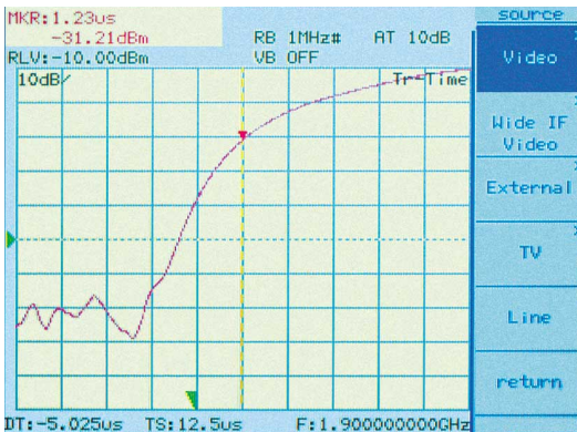
High-speed time-domain measurement (TS = 12.5 \mu s)
